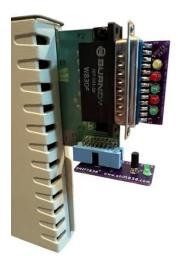
This program tests the ROM and both the serial and parallel ports. If an error is detected, the program stops and a diagnostic error message is displayed.
