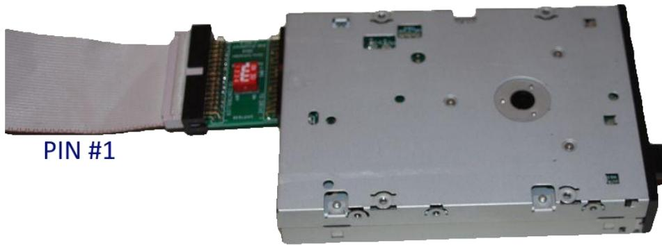
Step 5: Reinstall floppy drive ensuring the 838 Drive Select board is secure and does not touch any metal or conductive material.
